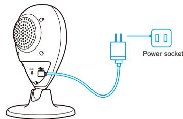
2. Press reset button for 5 seconds to hear the warning tone then release the button, wait for camera yellow and blue led lights is flashing alternately.
